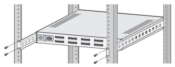
Figure 7. Securing Rear Support Rails to the Mounting Rails
